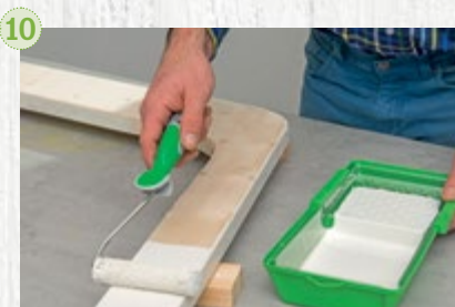
10. So the whole furniture piece does not get too colourful, a more subtle colour is recommended for the sides; here Osmo Wood-Wax Finish 3172 Silk was used. Open the finish, stir well and pour into the tray insert. Spread evenly onto the table sides with Osmo Microfibre Roller or Osmo Flat Brush.
