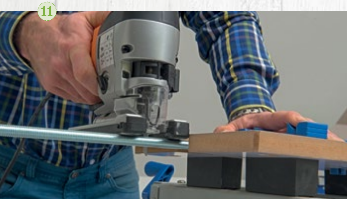
11. Threaded rods give the table sides more stability. Fix these in a vice or the clamping jaws of your workbench and shorten them to the appropriate length. Cut the four aluminium pipes to a length of 50 cm; these are used as covers for the threaded rods.
