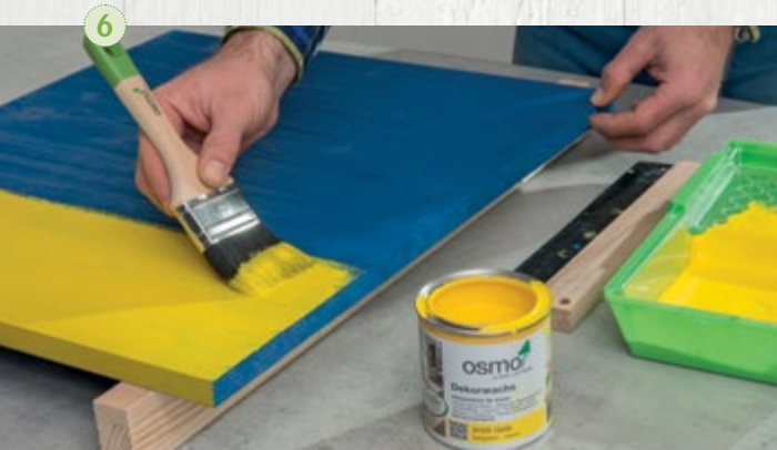
6. After thoroughly stirring, pour Wood Wax Finish in the second colour into the replaced roller tray insert and coat the surfaces like the base colour.
