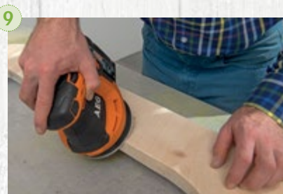
9. After cutting the panels, round off the edges with a sander or by hand and smooth surface with medium and fine grit sandpaper.
