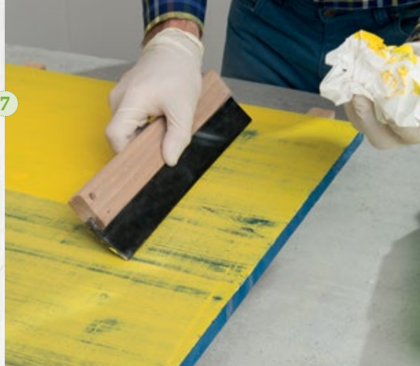
7. Now you have to act fast: Before the second colour dries, wipe away the second coat with the rubber scraper. Make sure to clean the scraper between laps. The base colour is now visible on the raised surfaces and second colour stays in the grooves. Allow the finish to dry for another 24 hours.
